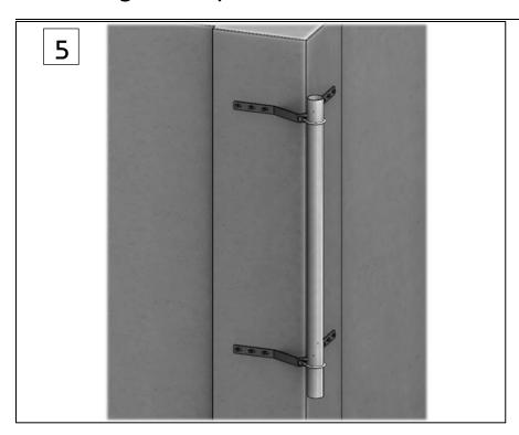
The tightening torques recommended in this mounting description presupposes bolts, threaded rods and nuts in delivery state. Nuts are to be lubricated before assembly.
