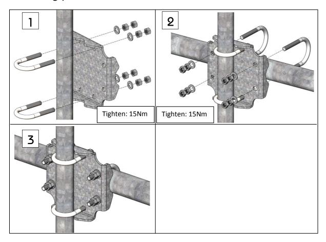
The tightening torques recommended in this mounting description presupposes bolts, threaded rods and nuts in delivery state. Nuts are to be lubricated before assembly.
