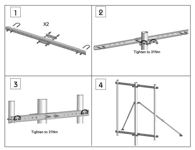
The tightening torques recommended in this mounting description presupposes bolts, threaded rods and nuts in delivery state. Nuts are to be lubricated before assembly.
